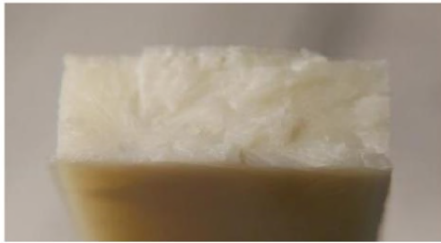
Close-up on the fracture of a 3D printed LUVOCOM 3F PA HT
