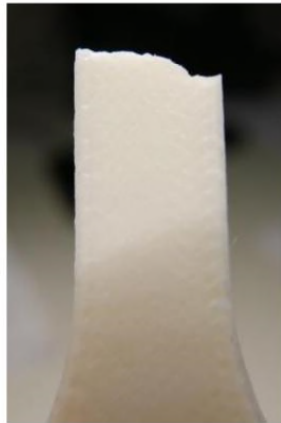
Close-up on the fracture of a 3D printed LUVOCOM 3F PA HT
